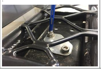
Remove the 2 capscrews securing the roof rack to the mounting bracket.
