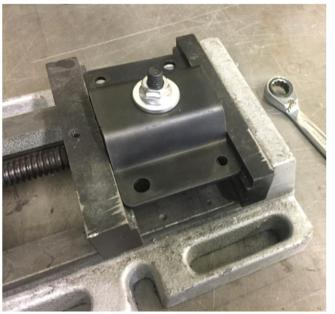
Place the bracket into a vice. Tighten the M8 nut against the washer to pull the knurled stud into the bracket.
